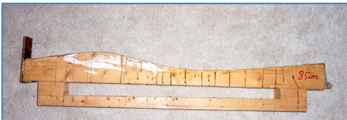
The first template is use to draw on a pine fir the front anatomy of slat.
