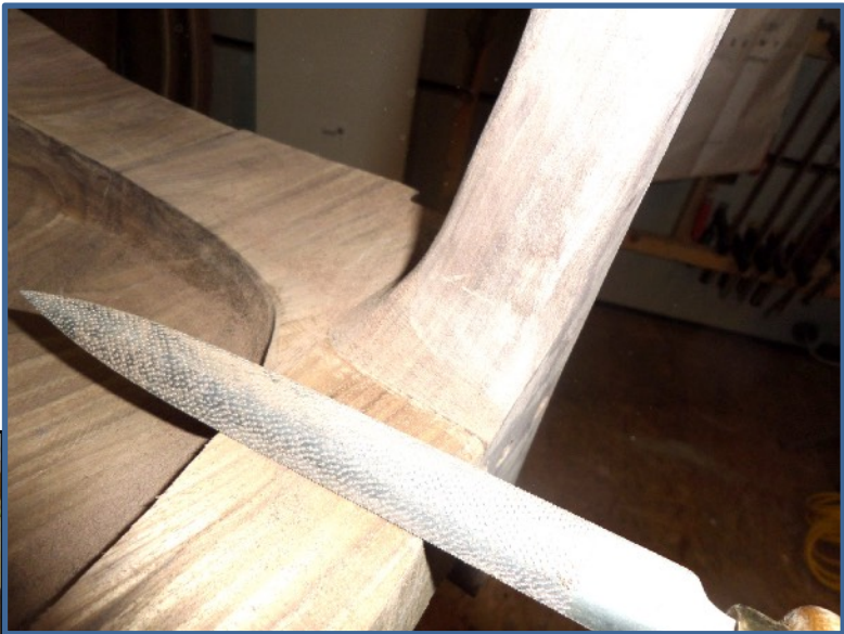
Lateral side seat can be resected, shaping can start, here Auriou chair rasp.
