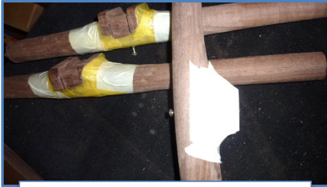
First stage : seat front feet and rear posts.
