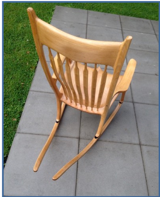
My preference, concave seat, hollow armrest, located lower on the seat, inclined front foot, 4° rear post.
