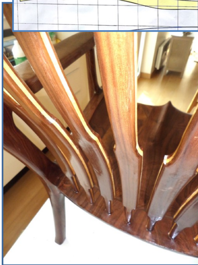
Laminated slats combining a layer of ash between two layers of walnut.
