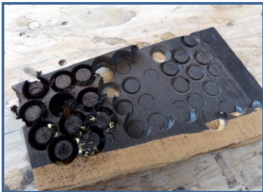
Some ebony for plug, inserted as dowel on screw heads.
