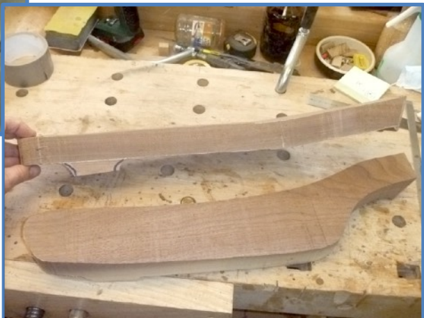
The hollow is traced to the posterior third, on a perfectly square block 5.5 to 6 cm thick. The cut pieces are fixed, with gray tape, to maintain stability on the bandsaw.
