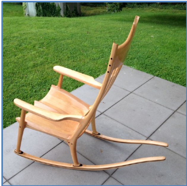
Beech Rocking-Chair , wenge insert, laminated slats, with « horn »
