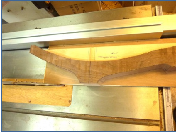
90 °cut of the anterior surface of the foot in preparation for making the tenon, 90° from seat.
