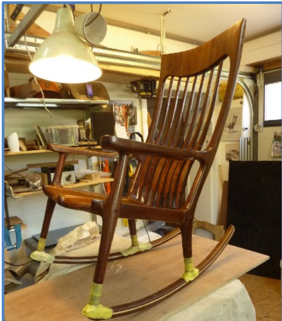
4th stage : gluing of the rockers AFTER SEAT BALANCE and first finishing layer.
