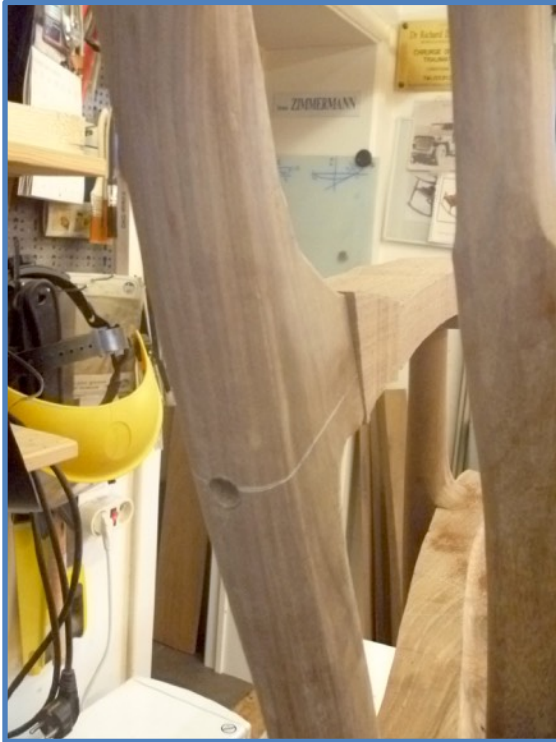
Laying dominoes : Screw in place tight, the internal face is flattened, a line in pencil is drawn, after dismantling a domino 20x8X40 mm, is done, making the mortise on each separate piece as usual.
