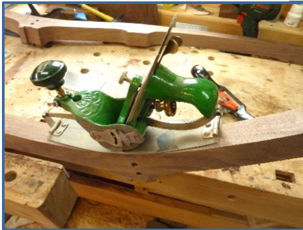
The foot is rounded back with Planer No. 113 or similar, reduced to 37 mm in thickness with band saw , except at the reserve level of the headrest and seat.
