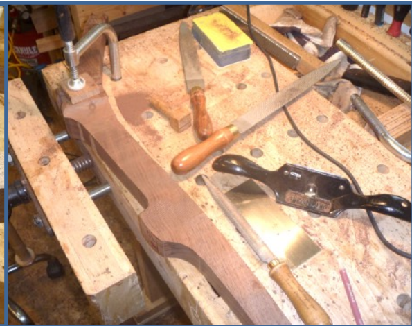
The foot is rounded back with Planer No. 113 or similar, reduced to 37 mm in thickness with band saw , except at the reserve level of the headrest and seat.
