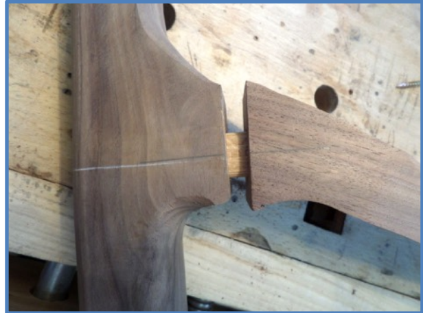
Laying dominoes : Screw in place tight, the internal face is flattened, a line in pencil is drawn, after dismantling a domino 20x8X40 mm, is done, making the mortise on each separate piece as usual.
