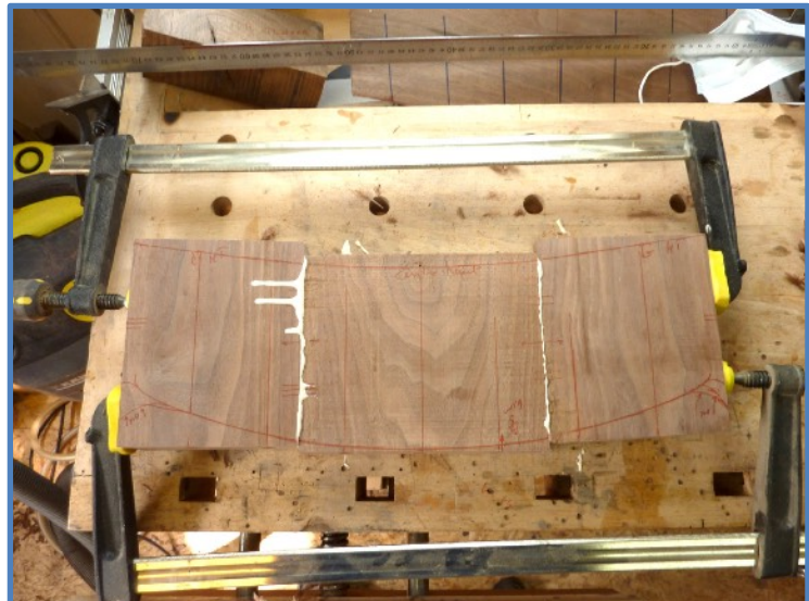
Three vertical blocks, are an alternative. The trouble is that the side must be shape parallel on table saw after gluing.
