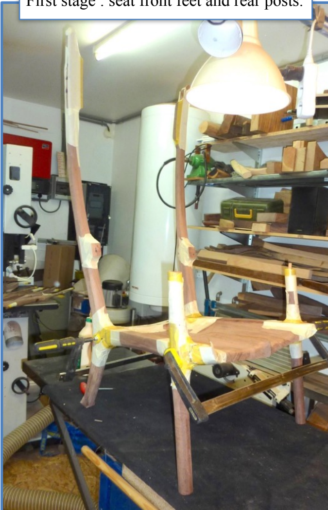
First stage : seat front feet and rear posts.
