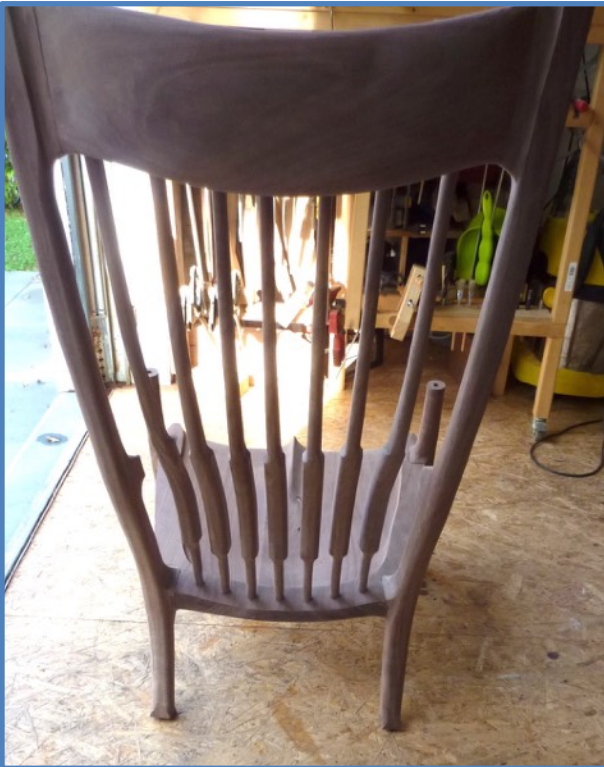
Each slat are refined and must fit up and down. Wood grain with « rifle butt » quality, can increase the aesthetic effect.
